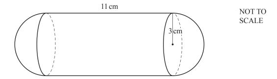
The diagram shows a solid made from a cylinder and two hemispheres. The cylinder has radius 3 cm and length 11 cm. Each hemisphere has radius 3 cm.
